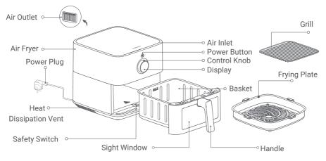
Notes: 1. The silicone rubber on the frying plate is made of high temperature resistant food-grade materials to prevent the edges of the frying plate from scratching the coating of the basket and to improve the stability of the frying plate. Do not remove the silicone rubber from the frying plate.
